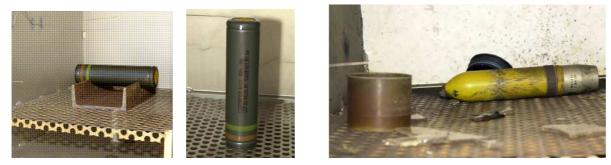
Figure 10: 40 mm cartridge before and after SCO test
