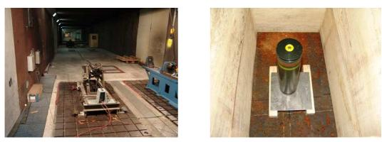
Figure 7: Weapon used for BI test and 40 mm ammunition before test
