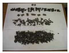
Figure 13: Fragmentation of 40 mm cartridge (static firing test)
